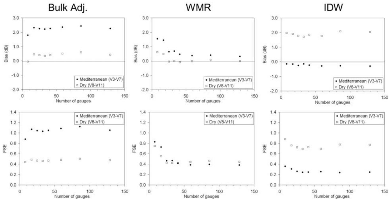
**Figure 7.** Effect of number of gauges in the training data set on bias and FSE for the two groups of climate regimes (Mediterranean and dry) and for the two radar estimate methods (bulk adjustment and WMR).
