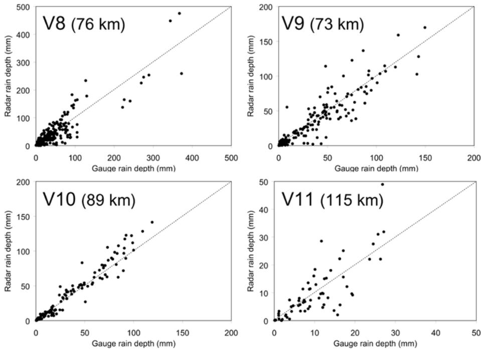
**Figure 6.** Fit between accumulated rain depth over rainfall periods derived from gauge and from radar for the four dry climate validation areas (V8–V11). Mean distance from radar is indicated in parentheses.
