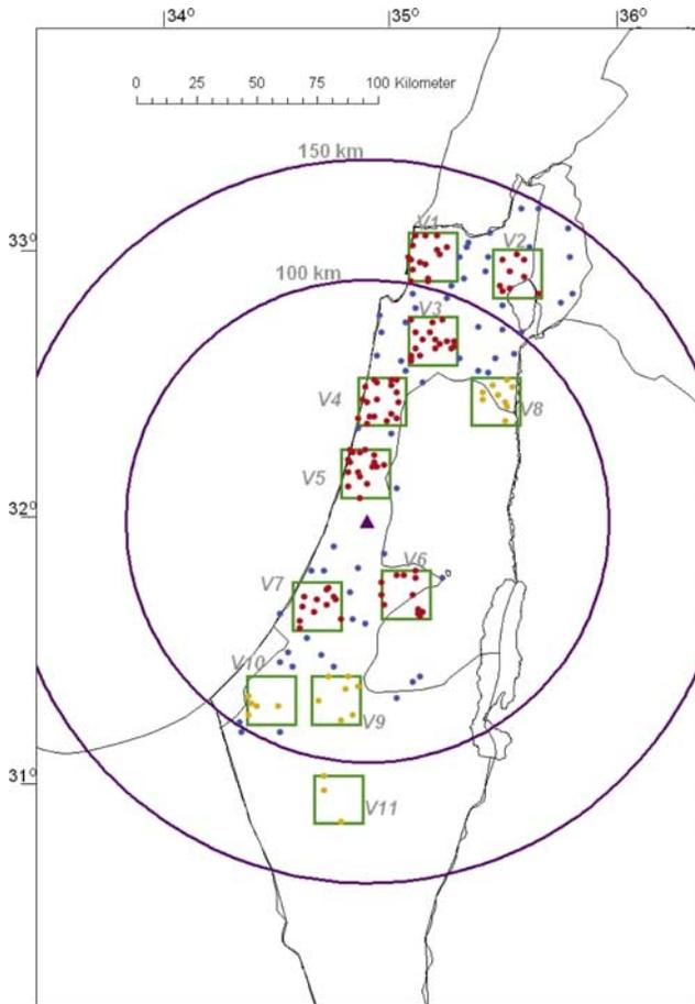
**Figure 2.** Rain gauges (solid circles) and the eleven validation areas of  $20 \times 20 \text{ km}^2$  size (marked by V1–V11). Radar location is marked by a triangle, and the 100 and 150 km radiuses are indicated.
