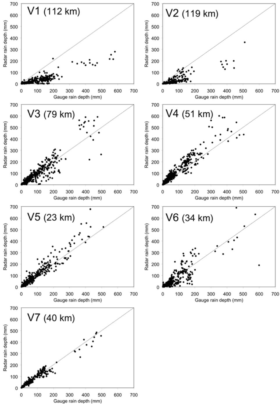
**Figure 5.** Fit between accumulated rain depth over rainfall periods derived from gauge and from radar for the seven Mediterranean validation areas V1–V7. Mean distance from radar is indicated in parentheses.
