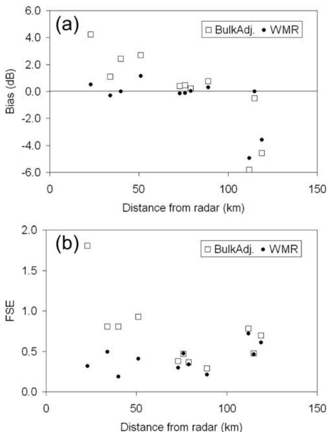
**Figure 4.** Errors (weighted averages) in terms of (a) bias and (b) FSE of radar estimates as a function of distance from the radar for the bulk adjustment and WMR methods.
